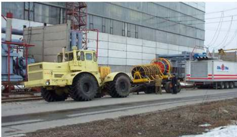
Fig. 2.1. Mobile emergency diesel-generator station, Kola NPP
